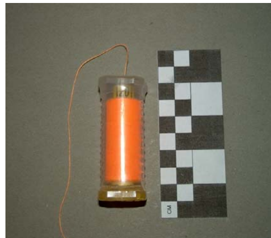
Figure 2.7.4. Trailer. Simply a standard roll of 200 meter cotton thread glued to the bottom of a plastic cylinder. The cylinder was then glued to the carapace and the thread tied to a tree or so. As the tortoise walked the thread was pulled out of the cylinder.
