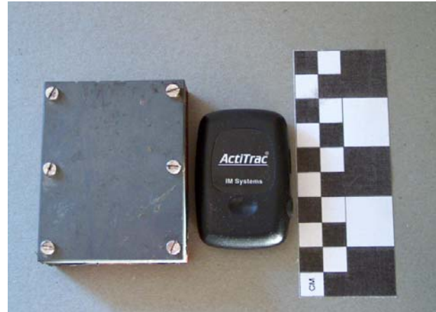
Figure 2.7.3. ActiTrac (middle) and custom made PVC casing (left). The casing was made of two pieces held together by six screws. Data from the ActiTrac could then be downloaded at any time simply by unscrewing the top piece. Scale bar to the right (small square = 1 cm)
